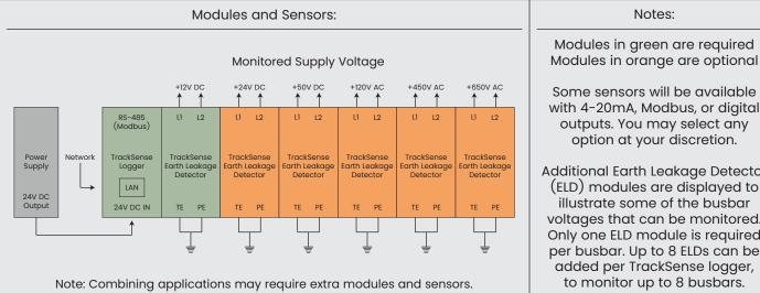
Below is an example wiring block. Wiring in practice may vary depending on requirements.
