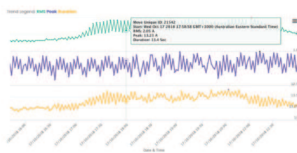
Asset trend view for predictive alerts and monitoring gradual performance degradation
