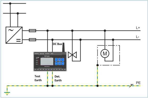
3.2.2.3 Monitoring of AC/DC Control Circuit
